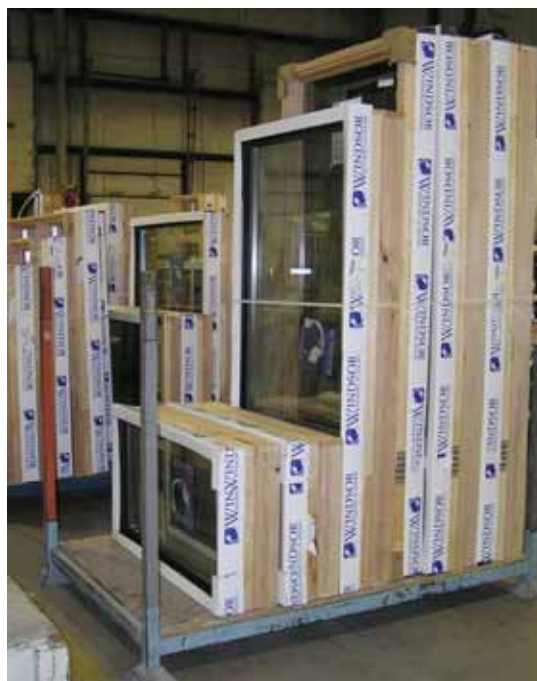
Windsor packages its windows in cardboard sleeves. They are held in place with banding during transport.
